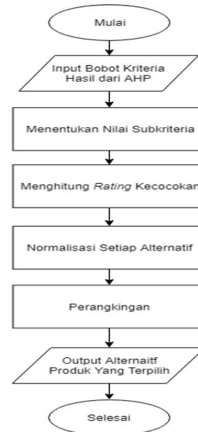
**Gambar 4.** Diagram alur perhitungan SAW
